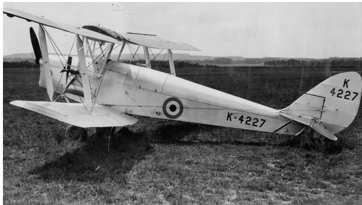
Figure 2.1: de Havilland DH82B Queen Bee [8], the first radio-controlled drone
