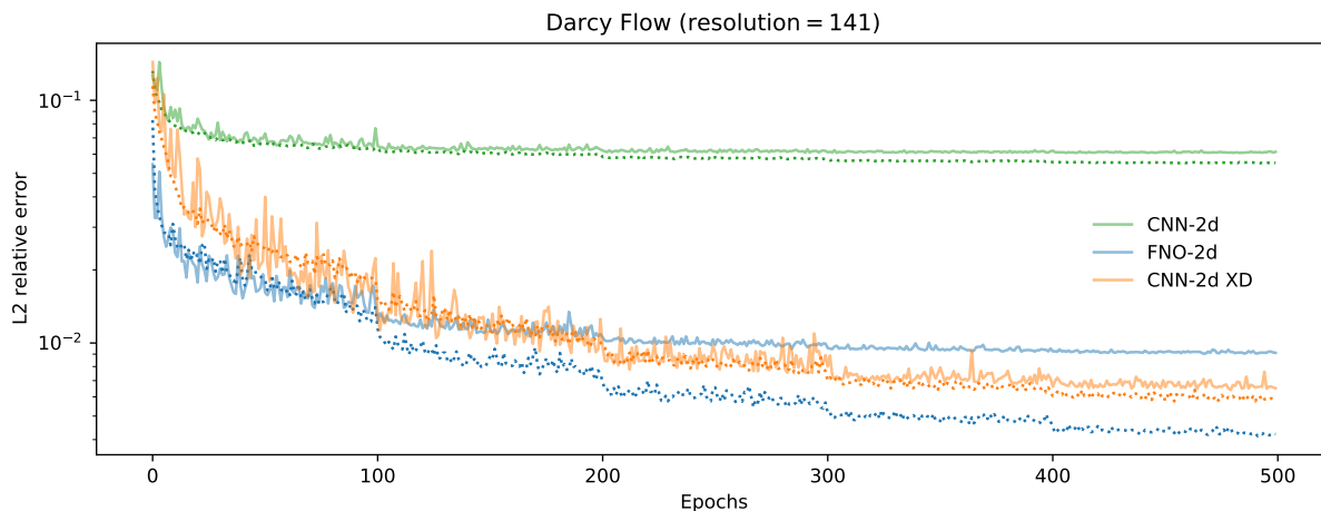
Figure 10.10: Training curves (dotted) and test curves (solid) on Darcy Flow at resolution 141, showing better generalization of XD-operations.
