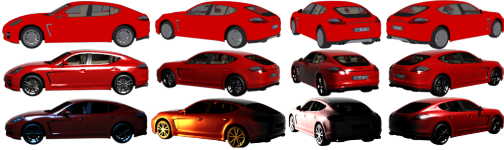
Figure 4.11: We evaluate the effect of render quality by creating 3 different conditions. The basic case uses simple object material, and ambient lighting (top row). Our intermediate setup has complex material and ambient lighting (middle row), and the sophisticated case has complex material, and directional lighting whose location, color, and strength are randomly selected.
