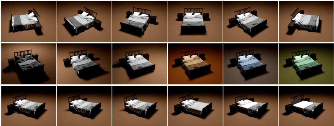
Figure 4.3: Rendered images of an IKEA bed. Generating synthetic data allows us to sample image properties in a controlled way. The top row shows sampling of viewpoint angle. In the middle row we sample lighting conditions, and in the bottom row occlusions by controlling the placement of night stands, and linens.
