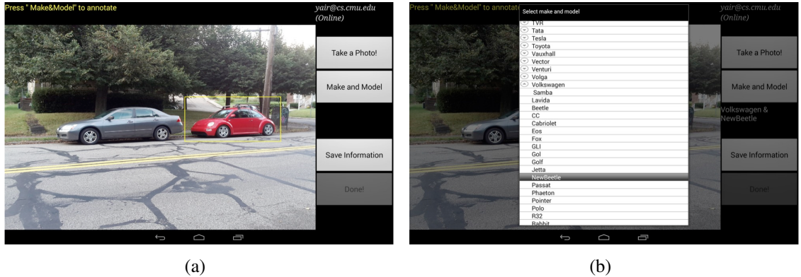
Figure 7.1: Screen shots from the CarSpotting annotation android application. Users can photograph cars in their surroundings, and annotate them with their make and model. Using a small team of volunteers we have collected a detailed dataset of about 3,000 images.
