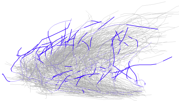
Figure 3.8: Outliers from Lee et al. shown in bold blue sections. Non-bold blue sections correspond to trajectory sections that are not anomalous for trajectories that contain at least one anomalous section.
