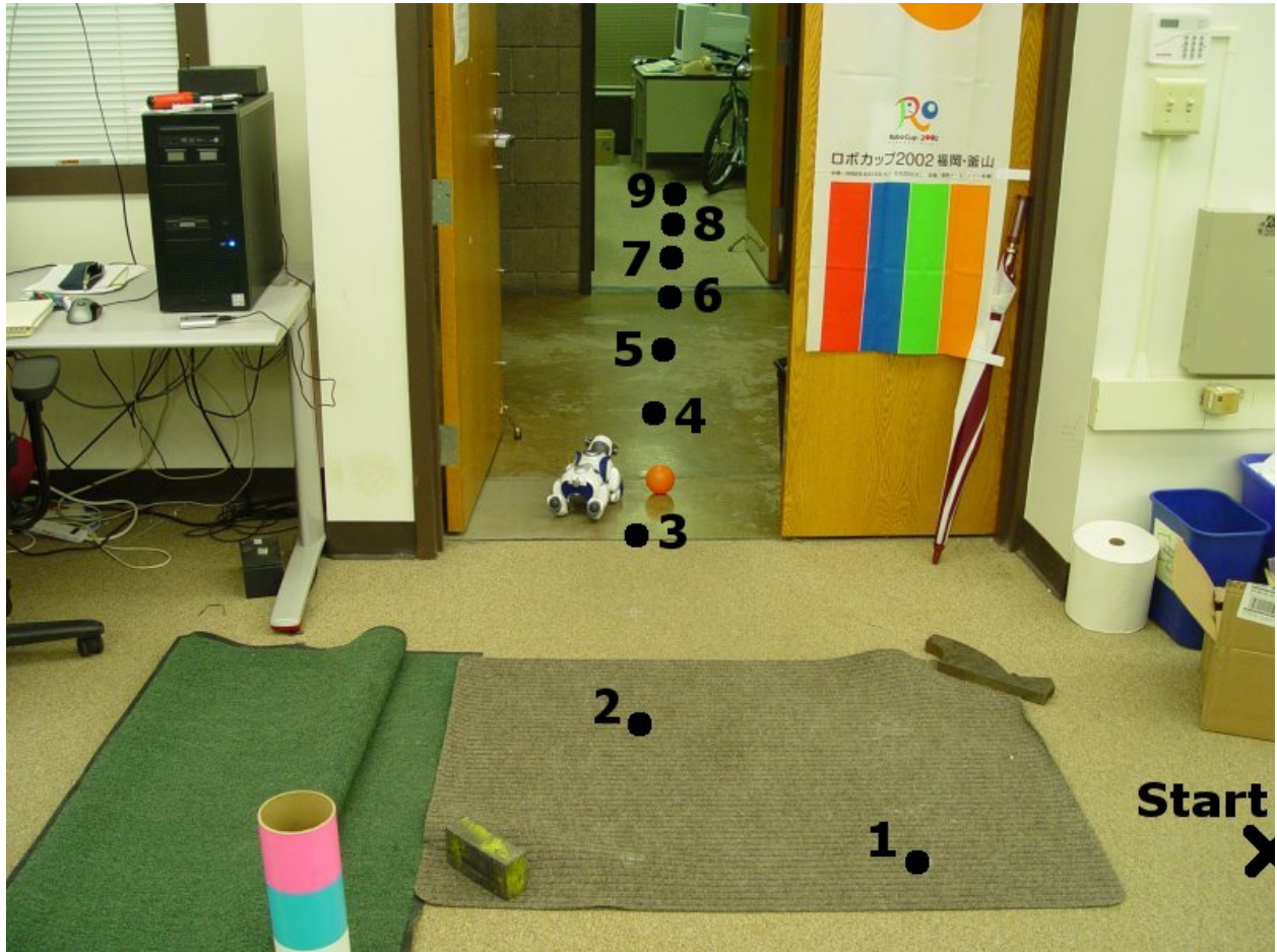
Figure 6.14: Setup for the ball chasing task. Each waypoint is marked in the image with a black dot and a numeric identifier. The actual waypoints were marked with clear tape so as not to interfere with the vision of the robot. The robot and ball are visible in the picture between waypoints 3 and 4.
